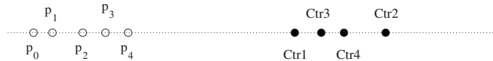
Fig. 4. A point may be moved in each rounding but all the displacements are in the same direction.
